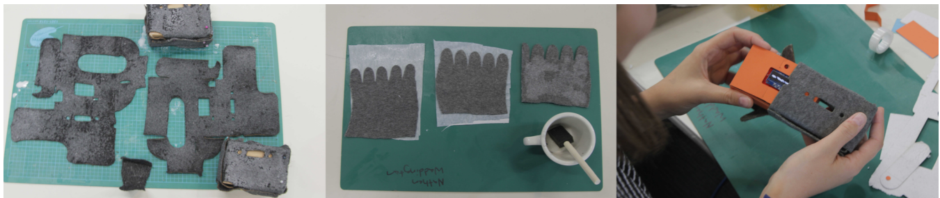
Figure 8. Our experiments with the soft enclosure included iteratively resizing the original lasercut file, stiffening the fabric using interfacing and applying fabric stiffener on the flat (pre-lasercut) and assembled (post-lasercut) enclosure. © 2018 Everyday Design Studio
