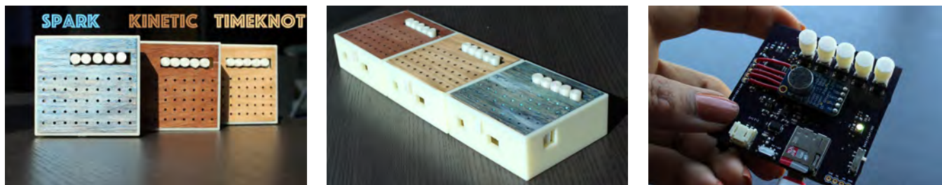
Figure 1. Left: The three devices of FamilyStories. Middle: All inputs and switches shown including On/Off and buttons for record, play, and share. Right: The interior Printed Circuit Board (PCB) designed to easily fit in one hand.
