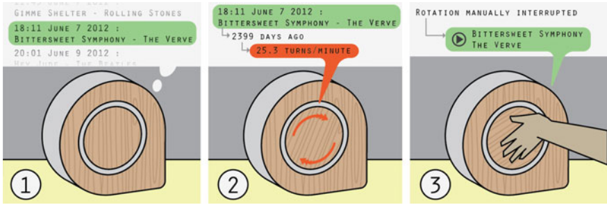
Fig. 4 (1) Olly’s algorithm has a ‘success’, and it randomly selects a specific listening instance from its owner’s Last.FM library; in this case, the song Bittersweet Symphony that was listened to on 18:11 June 7, 2012, is selected. (2) The internal disk begins to rotate indicating that a song is availability to be played; in this case, the listening instance is quite old which causing the disk’s rotational speed to be quite slow. (3) The user notices the rotation and manually spins the disk to trigger the song to play
