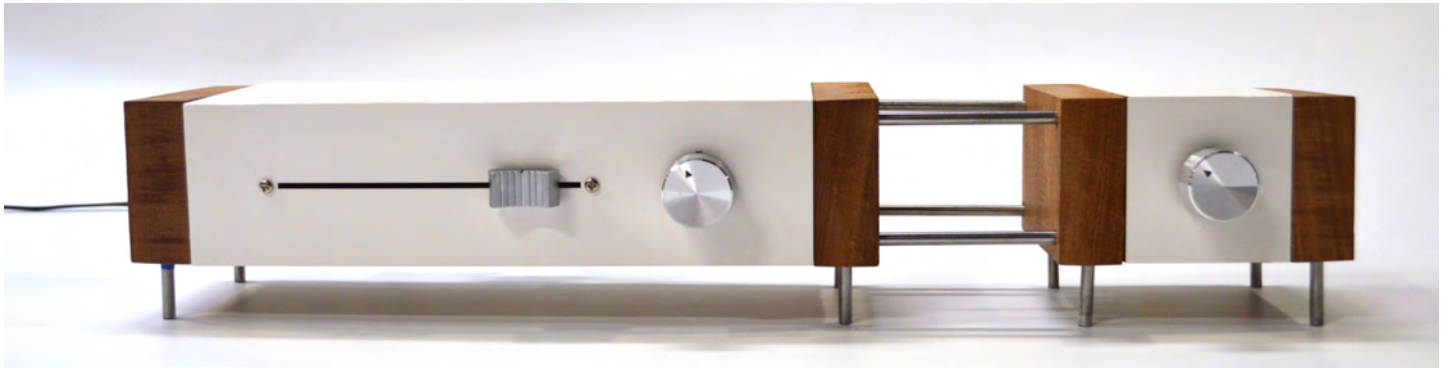
Figure 1. Drawing on a user’s archive of digital music listening history metadata, OLO Radio embodies the lifetime of music a user has listened to. The motorized linear slider and 3-switch knob exhibited on the left cabinet enable the user to explore, interact, and listen to music from their past across different timeframe modes; the rightmost knob controls on/off and volume.
