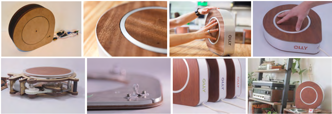
Figure 2. Olly. Top (Left to Right): T1. An early functional MDF prototype; T2. Rich veneer wood grains move in and out of alignment as the internal disc rotates; T3. A pending song is played by spinning the rotating disc; T4. Olly can operate lying flat (or in any other orientation). Bottom (Left to Right): B1. MDF chassis with low-wear timing belt driving Olly’s rotation; B2. 5mm aluminum plate with boat-grade veneer epoxied to it; B3. Three Olly research products; B4. Design team member (Odom) living with Olly during testing.
