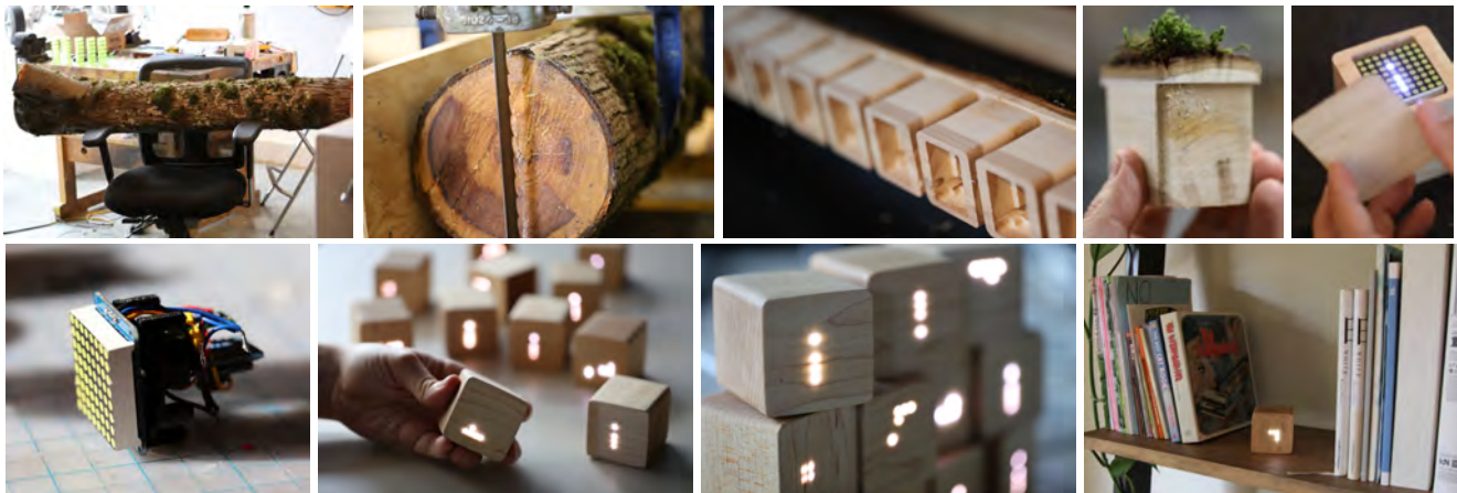
Figure 3. Slow Game. Top (Left to Right): T1. Log felled during a windstorm; recovered by design team; T2. Recovered log treated with beeswax and dried over months, then cut and planed; T3. CNC milled batch production of enclosures; T4. Early form exploration; elongated cube-like form with exposed bark and moss where mini USB power cable is inserted; T5. Affixing hand cut and then laser cut veneer to front face of final 5cm cube design. Bottom (Left to Right): B1. Custom design 3D-Printed chassis with tight integration of all components; B2.+ B3. Several Slow Game research products; B4. Design team member (Odom) living with Slow Game during testing.
