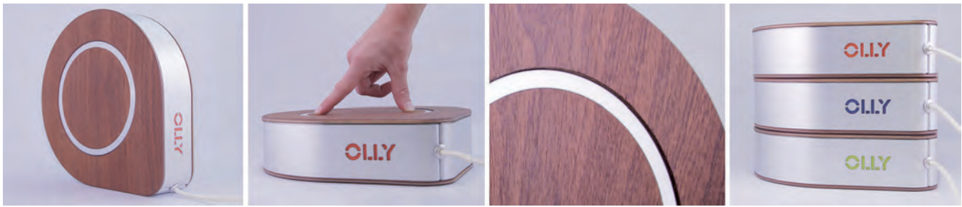
Figure 2: Left to Right. Olly can operate standing up (or lying flat); A pending song is played by gently spinning the rotating disc (pictured here when lying flat); Woodgrains move in and out of alignment as the disc rotates; 3 Olly research products deployed with participants.
