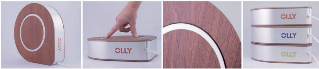
Figure 3. Left to Right. Olly can operate standing up (or lying flat); A pending song is played by gently spinning the rotating disc (pictured here when lying flat); Woodgrains move in and out of alignment as the disc rotates; Three Olly design artifacts.
