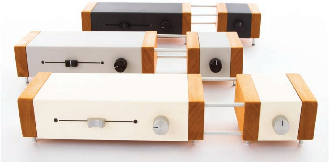
Figure 7. Drawing on a user's archive of digital music listening history, Olo Radio embodies the lifetime of music a user has listened to. The motorized linear slider and 3-switch knob exhibited on the left cabinet enable the user to explore, interact, and listen to music from their past across different timeframe modes; the rightmost knob controls on/off and volume.
