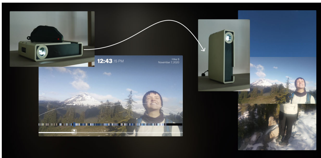
Figure 21: The accelerometer within the Explorer identifies when it is rotated between its horizontal and vertical orientations, and switches between the two projected UI states. When in horizontal mode only the eye-level PoV image is displayed, while in vertical mode the additional screen height is optimal to display all three PoVs.
