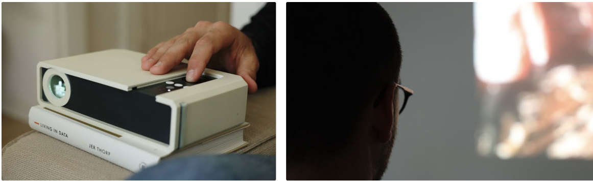
Figure 12: The Capra Explorer is roughly the size of a medium-sized hardcover book. It stores the archive of images and metadata, is the site of interaction and exploration, and projects onto a wall in the user’s home.
