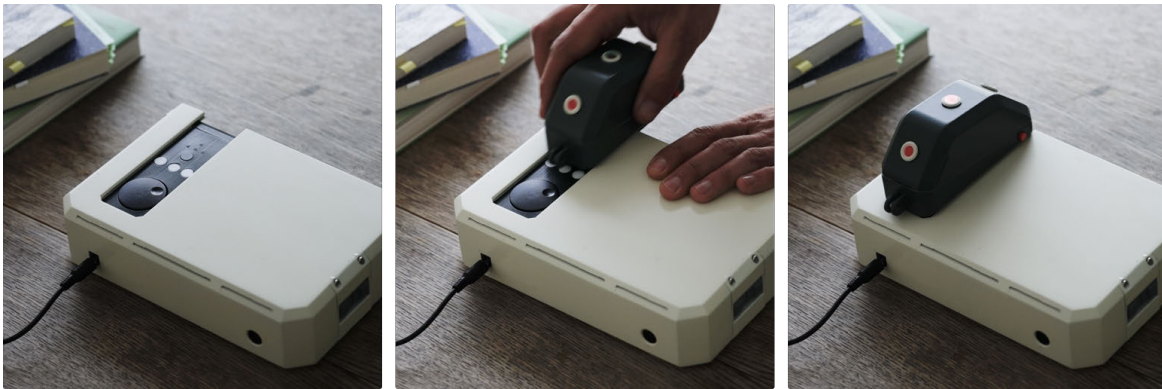
Figure 9: The Collector slides into the Explorer and renders the control interface inaccessible.
