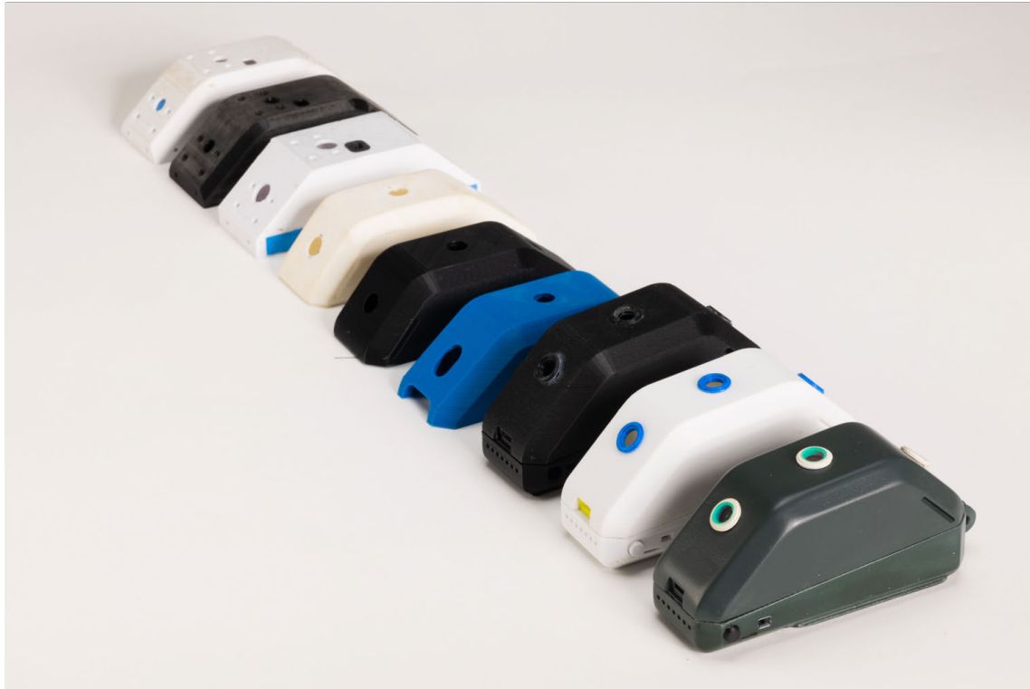
Figure 5: Numerous iterations of the 3D printed Collector enclosure were required to integrate three cameras and their associated hardware and lenses into a resolved form that was both small and light enough to wear comfortably on a backpack strap, and robust enough to survive hiking in the wild.
