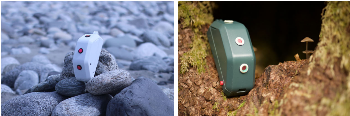
Figure 7: The Collector is easily detached from its mounting point, so that it can shift from capturing hyperlapses to timelapses and thus encode other than human perspectives within the hiking data.
