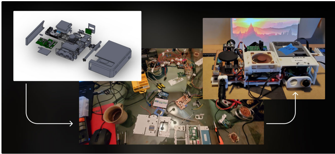
Figure 22: (left) Exploded CAD illustration of the Explorer showing some internal components. (center) In progress assembly of the Explorer with our custom PCB. (right) Collector unit test before being sealed in the enclosure.
