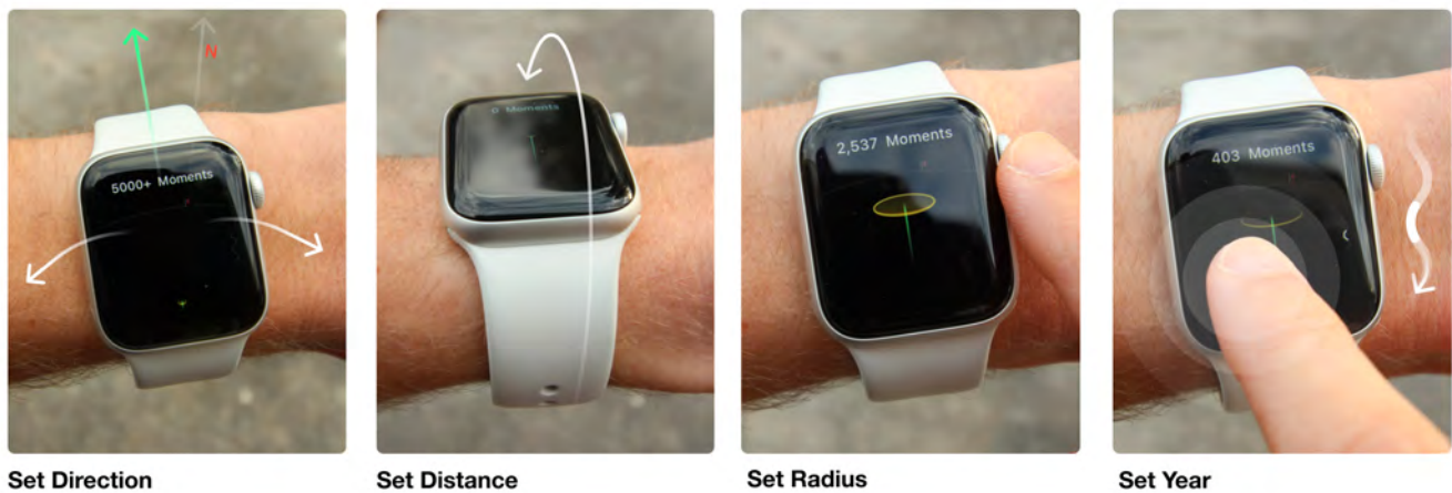
Figure 12: The interactions to adjust the direction , distance , radius , and year filters for Memory Compass
